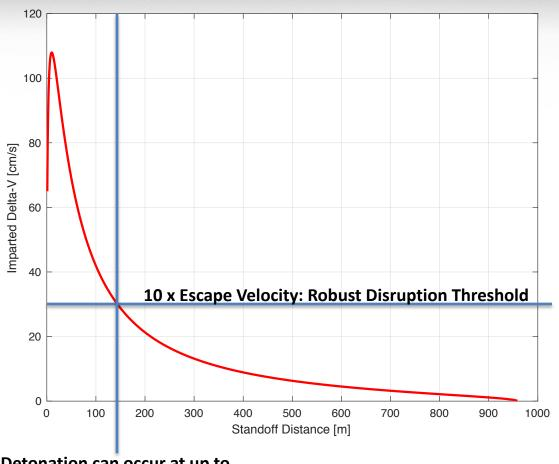
Detonation can occur at up to ~145 m from asteroid
